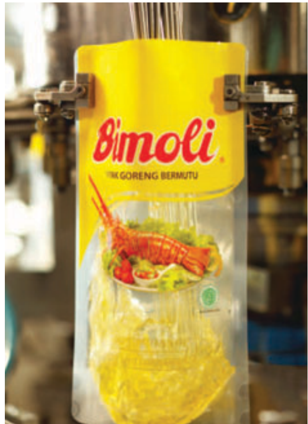
Filling of cooking oil into refillable package
